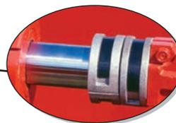
Threaded adjusting rods installed on the base end of wing cylinder serves to determine uniform depth during the field operations. The existing scale set in centimeters on the shanks allows to visualize depth of work.
