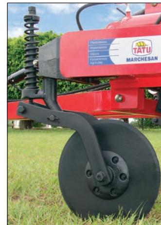
**18" Coultter Blades:** are used to cut and reduce volume of straw to avoid clogging.
