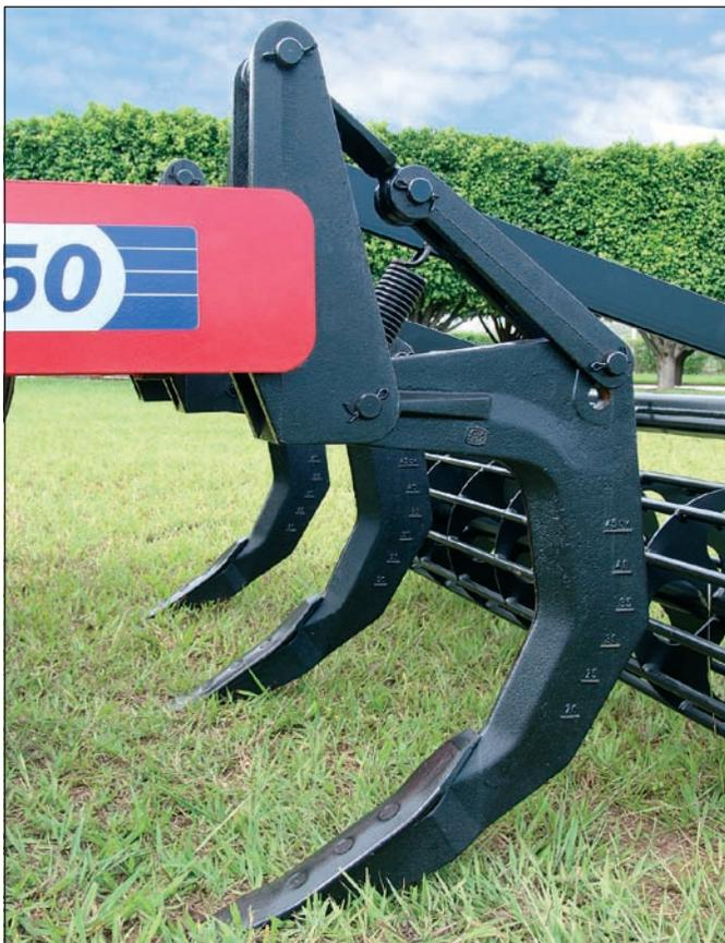
This system is spring loaded on each shank, when a rock, root or stump is hit, the shank will flip back and return to working position when the implement is raised. It does not require any cares for maintenance or adjustments due to its reduced dependence of the moving parts.
