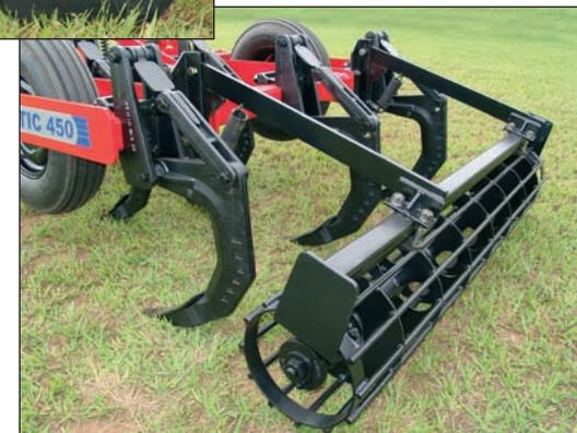
**Breaker Roller:** - used to reduce the lumps and make easy operation of other implements.
